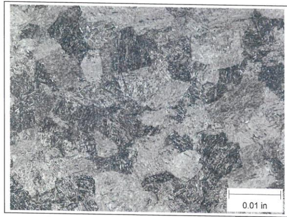
Yoke #2, x100 ASTM grain size 2.5
