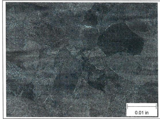
Hub, x100 ASTM grain size 2.5
