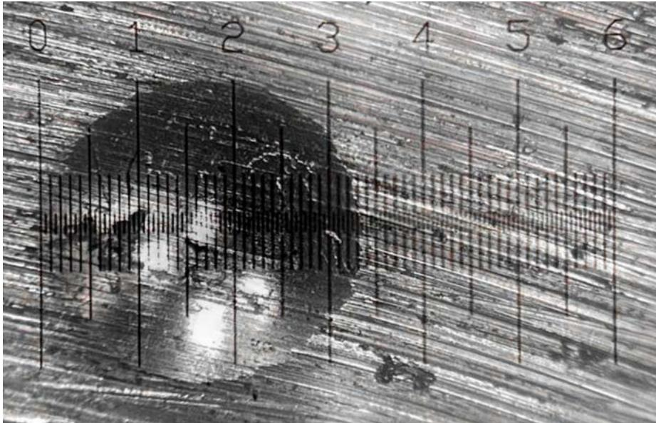
Figure 3. Measurement of Brinell hardness test indentation
