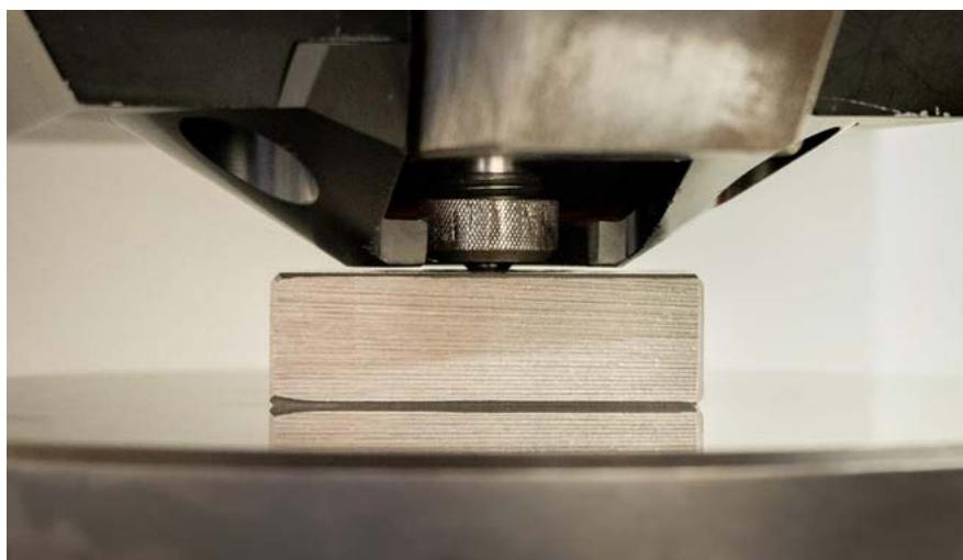
Figure 2. Close-up of a calibration-grade Brinell tester
