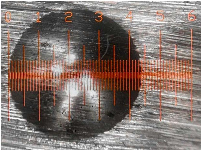
Figure 4. Measurement with improved microscope and well-illuminated graticule
