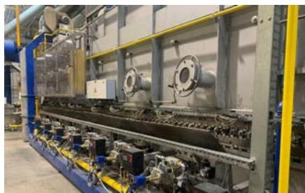
Indirectly heated roller hearth furnace
