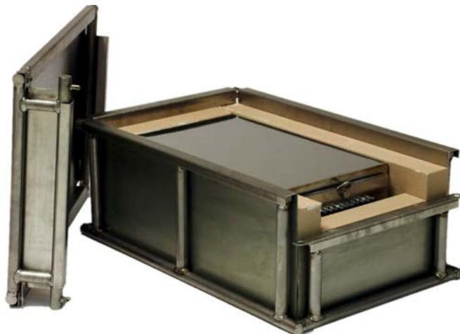
Figures 4. Phoenix<sup>TM</sup> thru-process temperature profiling system monitoring the core temperature of automotive parts in a traditional sealed gas carburizing furnace with integral oil quench. (left) System entering carburizing furnace in product basket. (right) Thermal barrier showing outer structural frame and sacrificial insulation blocks protecting inner sealed thermal barrier housing the data logger. (Source: Phoenix<sup>TM</sup>)
