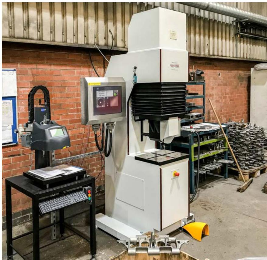
Figure 1. Heavy-duty Brinell tester in situ
