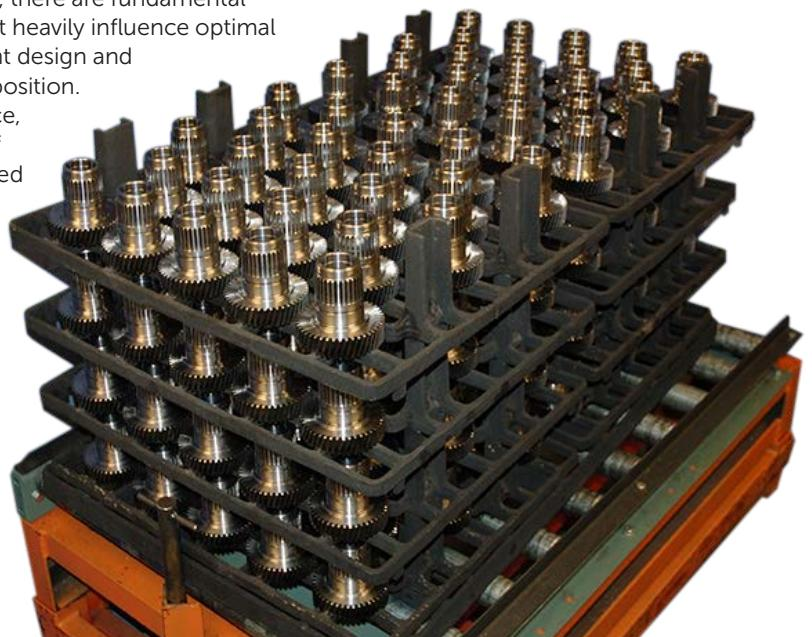
Figure 1. Cast tray and fixtures (Source: Castalloy Group)
