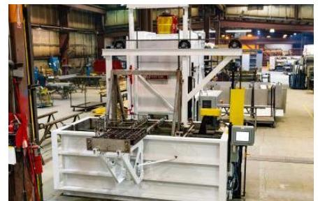
Horizontal quench system for aluminum solution treatment
