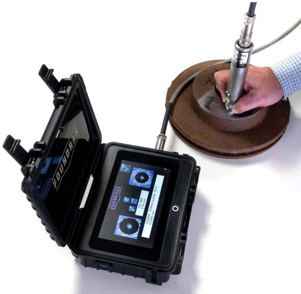
Figure 5. Latest version of the automatic microscope in action
