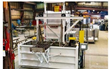
Horizontal quench system for aluminum solution treatment
